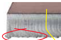
Result of torch-to-work distance too high
