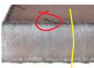
Result of slow speed and torch-to-work distance too high
